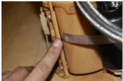
17. Place the fuel pump next to the factory pump basket and secure it loosely using the worm clamp. Be sure to aim the pump pick up towards the back of the car. This is where the mark you made on the fuel pump basket will come in handy.
