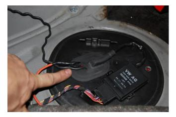
26. Connect the red power wire from the fuel pump and bulkhead assembly to the WHITE wire from the control box and the black ground wire from the fuel pump and bulk head assembly to a good chassis ground.
