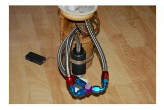
Please note: The fuel pump kits now ship with a stainless steel barb "Y" fitting with crimp clamps. This reduces clutter.
