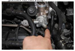
2. Using your Schrader valve core tool remove the valve core located inside the brass fitting that we just removed the cap from. The core must be turned in a counter-clockwise motion to be removed. If it is too difficult to remove the valve core, simply remove the entire brass fitting from the fuel pump housing using a 13mm wrench. Then remove the valve core and reinstall the fitting on the pump.
